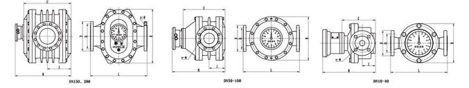
• Dimensions and weight of cast iron type (B dimension is the dimension of the configuration A or J1 counter
