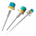
The vibration is generated by the magnet and electromagnet set in the inspection tube, and the difference of the current flowing through the electromagnet is checked when there is a powder object and there is no powder object, and the inspection signal of the powder object is output. In case that the inspection part is not covered by powdery objects, etc.:
